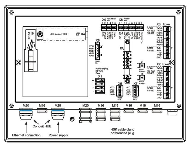
Any cable glands at the operator interface that are not required **<u>MUST BE</u>** replaced by threaded plugs so that the opening in the housing is covered.
